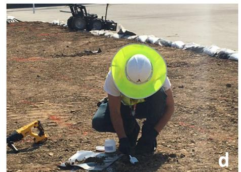
*The fieldwork to retest the soils in the trench sites, includes breaking up the asphalt (a), excavating (digging up) the soil (b), laying the soil on radiological screening yard (RSY) pads (c), and scanning and sampling the soil from the RSY pads. Photos from EPA field oversight (September 2020).*
