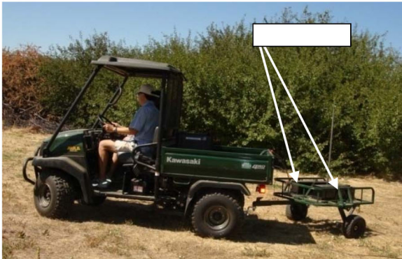
Figure 1: RS 700 Mapping system (towed array)
