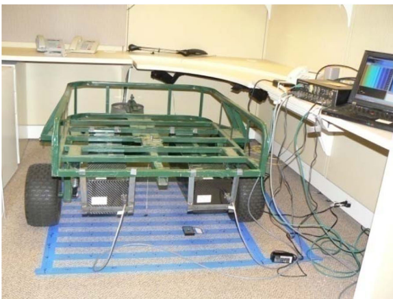
Figure 2: RS 700 Electronics and detectors on trailer
