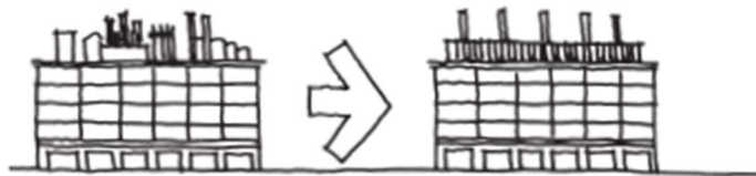
Fig. 45 Screen Mechanical Equipment
