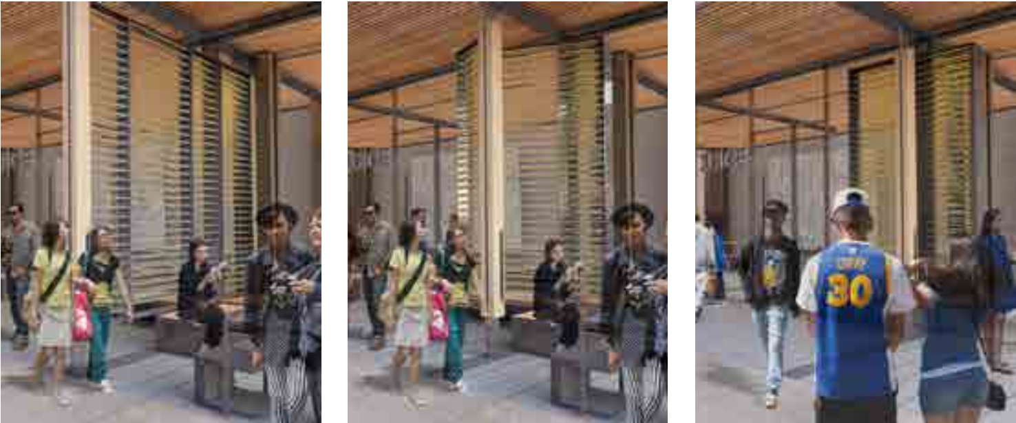
Windbreak Element Operability: The windbreak elements are designed to fold into the building, allowing for modulation of the width of the sidewalk.
