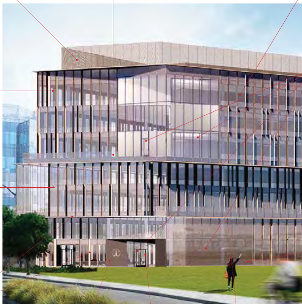
Shadow Box: Glass Coating to Match Upper Level North Glazing Solarban 60 Custom Paint for Shadow Box
