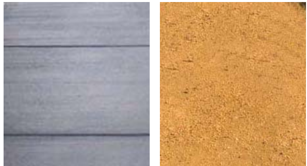
01 C.I.P. Concrete Paving 02 Stabilized Crushed Stone Paving
