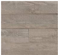
01 Board Formed Concrete
