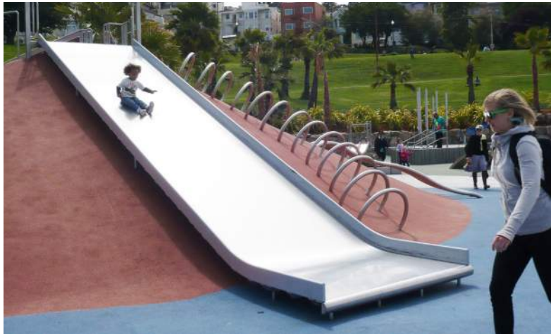
F9 Slide Custom stainless steel embankment slide
