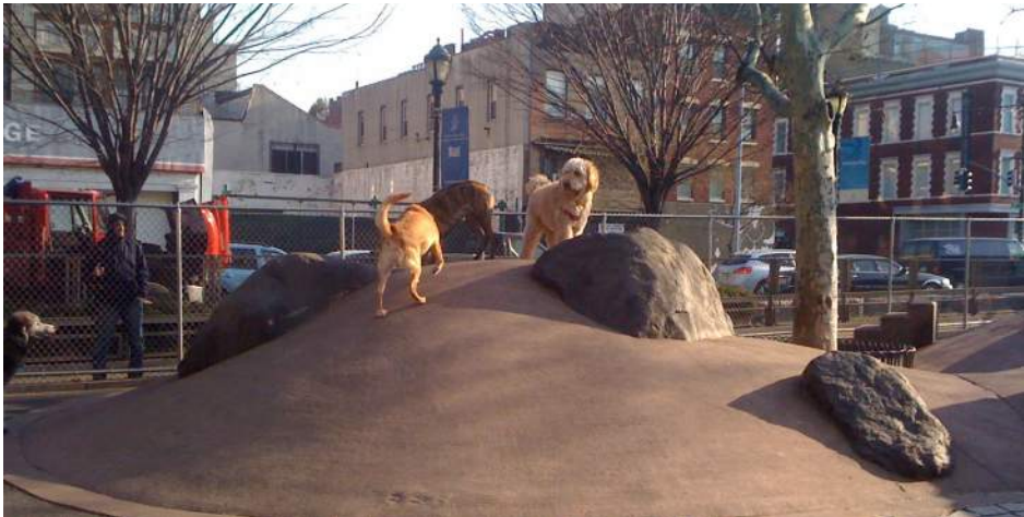
F8 Dog Park Boulders Glass fiber reinforced concrete
