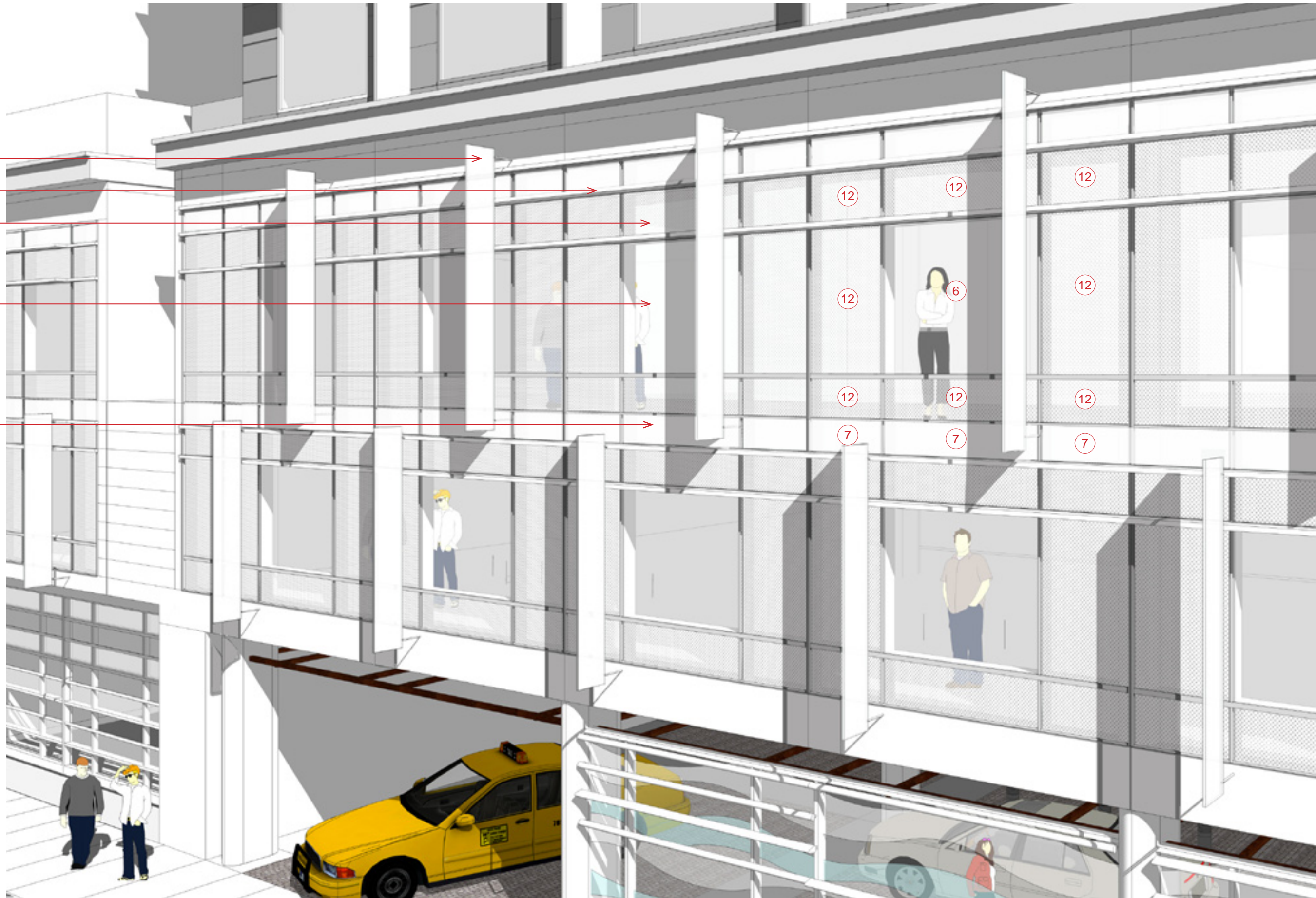
Schematic Design | Enlarged Tartan Window Wall at Podium with Vertical Solar Sunshades
