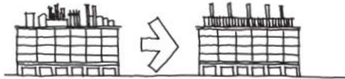
Fig. 45 Screen Mechanical Equipment
