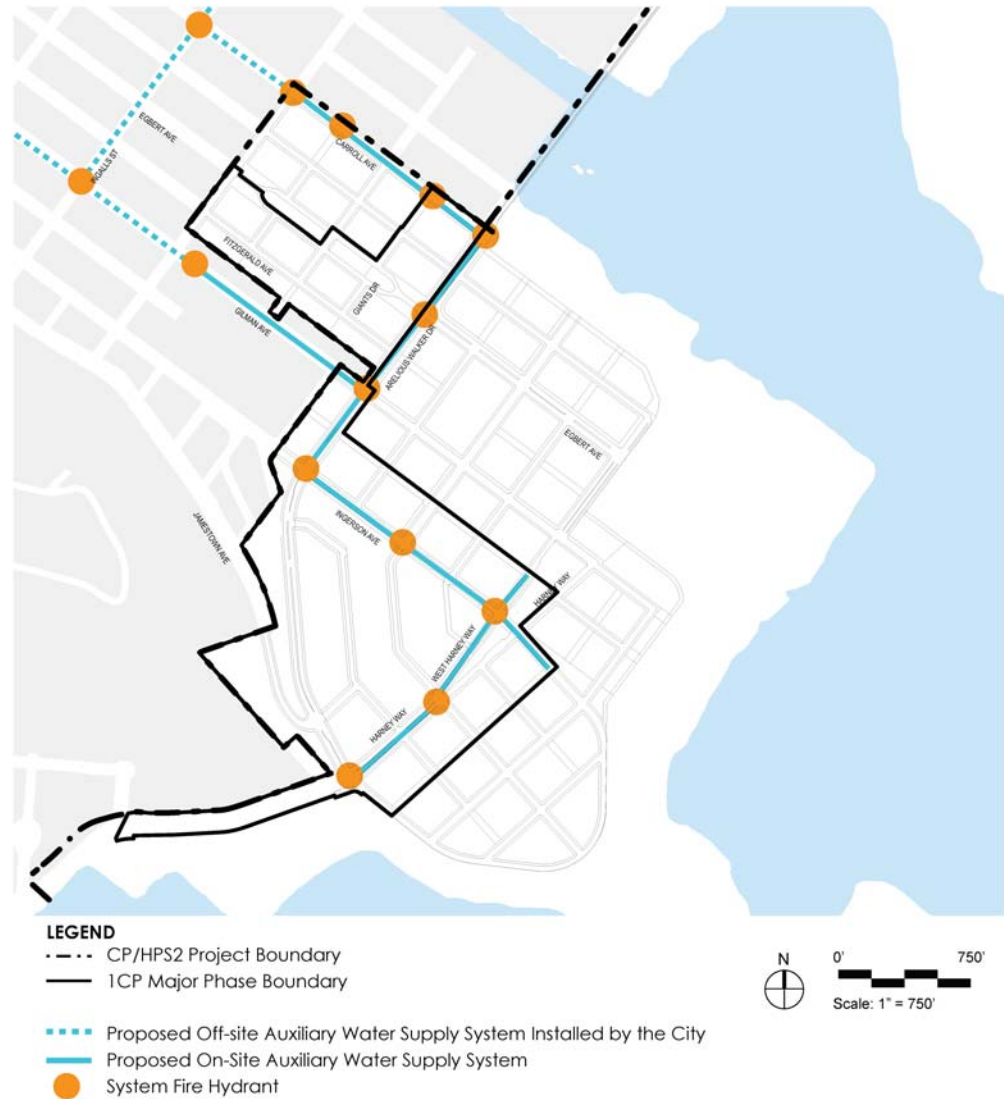
FIGURE 9.5: AUXILIARY WATER SUPPLY
