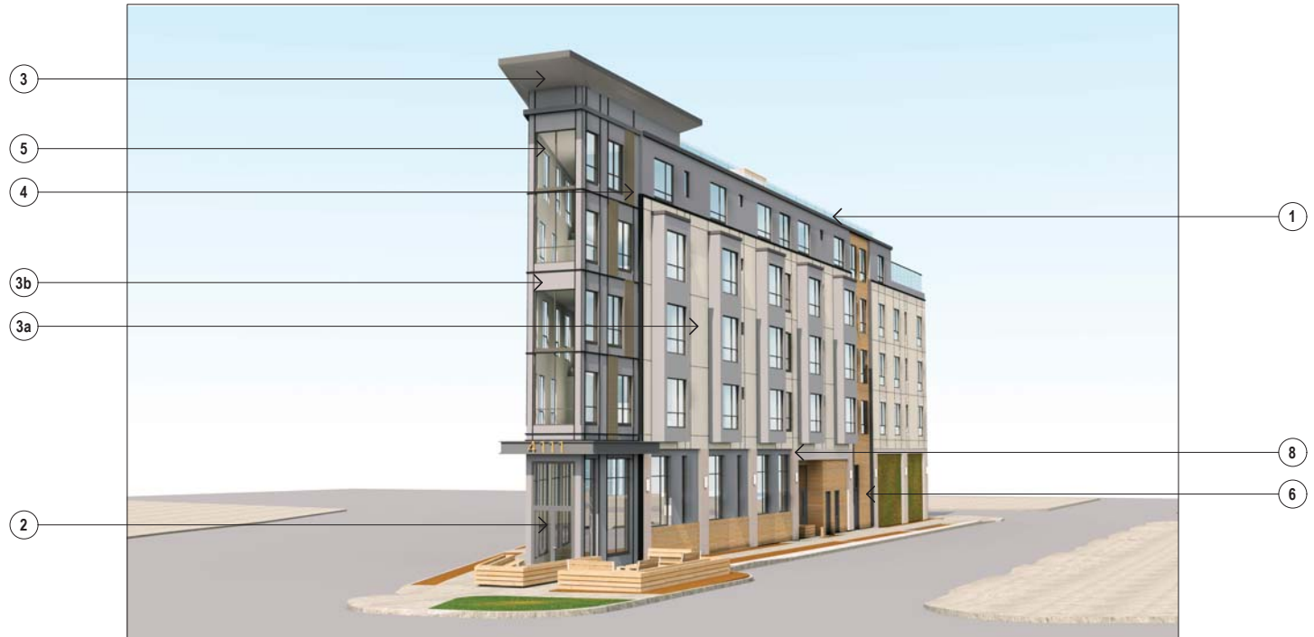
4 EXTERIOR ALUMINIUM SHEET SUN SHADING SYSTEM, BRONZED ANODIZED PERFORATED STAGGERED 16 GAUGE, ROUND HOLE, 3/32" HOLES ON 5/32" CENTERS, 33% OPEN AREA, BACK-LIT AT NIGHT
