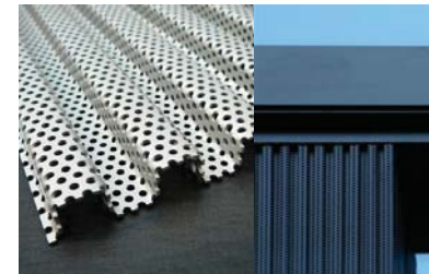
4 EXTERIOR ALUMINIUM SHEET SUN SHADING SYSTEM, BRONZED ANODIZED PERFORATED STAGGERED 16 GAUGE, ROUND HOLE, 3/32" HOLES ON 5/32" CENTERS, 33% OPEN AREA, BACK-LIT AT NIGHT
