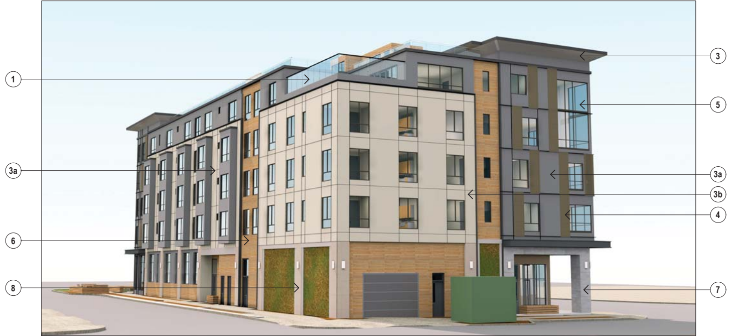
4 EXTERIOR ALUMINIUM SHEET SUN SHADING SYSTEM, BRONZED ANODIZED PERFORATED STAGGERED 16 GAUGE, ROUND HOLE, 3/32" HOLES ON 5/32" CENTERS, 33% OPEN AREA, BACK-LIT AT NIGHT
