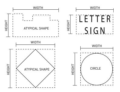
Figure 4.30a: SIGN AREA CALCULATION DIAGRAM
