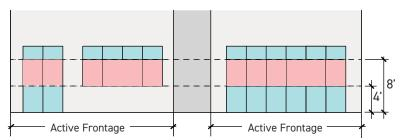
Figure 4.11e: GROUND FLOOR TRANSPARENCY CALCULATION
