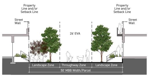
Figure 4.1e: TYPE 2 MID-BLOCK BREAK WIDTH (50')
