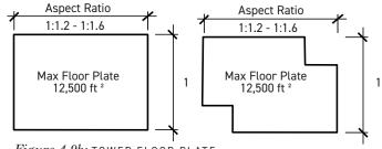
Figure 4.9b: TOWER FLOOR PLATE
