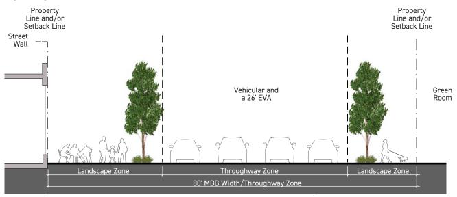
Figure 4.1h: TYPE 4 MID-BLOCK BREAK WIDTH (80')
