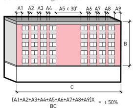
Figure 4.17b: UPPER FLOOR BLANK WALLS CALCULATION
