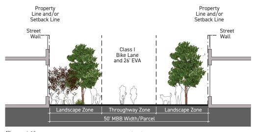
Figure~4.1f: Type 2A mid-block break width (50') with class I bicycle lane
