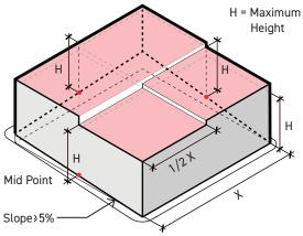
Figure 4.4b: BUILDING HEIGHT ON SLOPE
