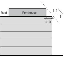
Figure 4.4f: PENTHOUSE STRUCTURE REQUIREMENTS
