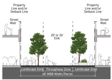
Figure 4.1c: TYPE 1 MID-BLOCK BREAK WIDTH (40') COMMERCIAL
