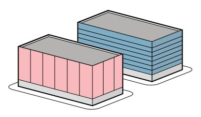
Figure~4.6d: block a (Vertical articulation and material color) BLOCK B (HORIZONTAL ARTICULATION AND MATERIAL COLOR)
