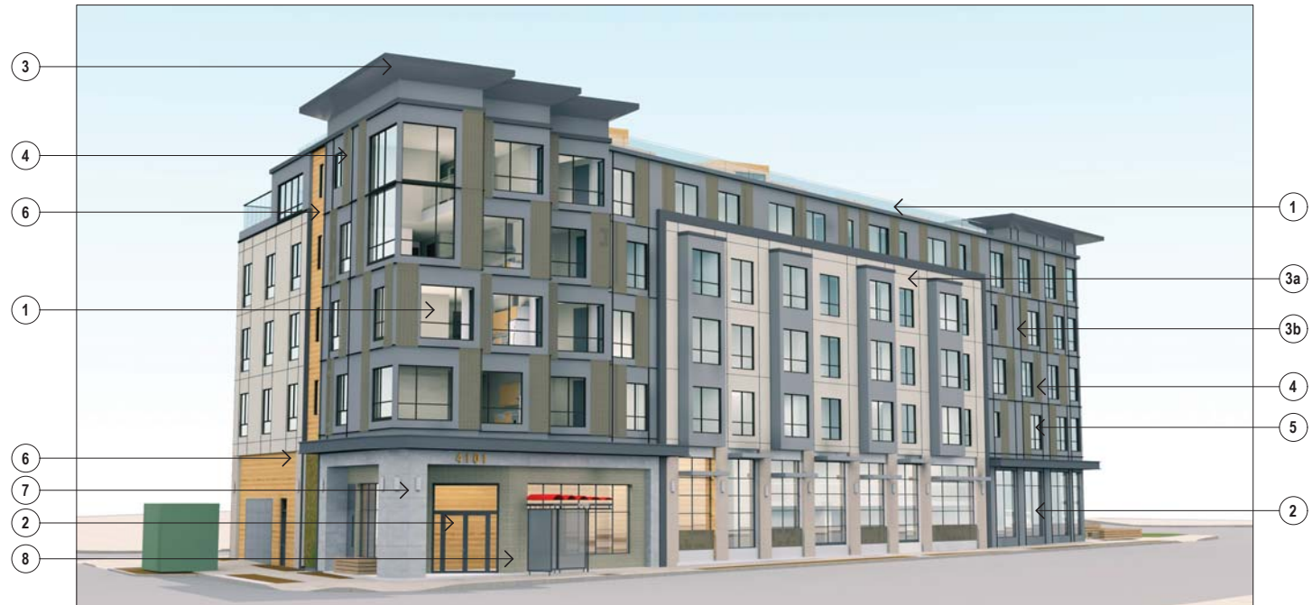
④ EXTERIOR ALUMINIUM SHEET SUN SHADING SYSTEM, BRONZED ANODIZED PERFORATED STAGGERED 16 GAUGE, ROUND HOLE, 3/32" HOLES ON 5/32" CENTERS, 33% OPEN AREA, BACK-LIT AT NIGHT
