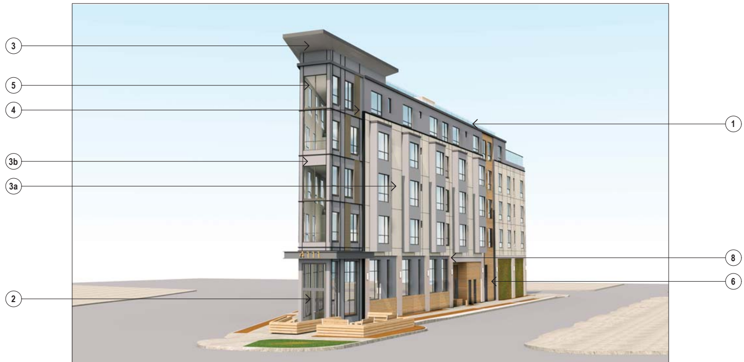
④ EXTERIOR ALUMINIUM SHEET SUN SHADING SYSTEM, BRONZED ANODIZED PERFORATED STAGGERED 16 GAUGE, ROUND HOLE, 3/32" HOLES ON 5/32" CENTERS, 33% OPEN AREA, BACK-LIT AT NIGHT
