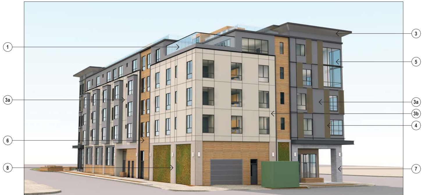
4 EXTERIOR ALUMINIUM SHEET SUN SHADING SYSTEM, BRONZED ANODIZED PERFORATED STAGGERED 16 GAUGE, ROUND HOLE, 3/32" HOLES ON 5/32" CENTERS, 33% OPEN AREA, BACK-LIT AT NIGHT
