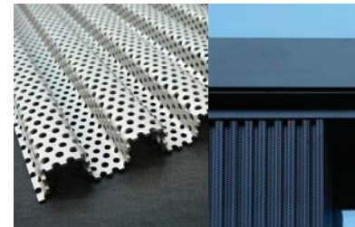
4 EXTERIOR ALUMINIUM SHEET SUN SHADING SYSTEM, BRONZED ANODIZED PERFORATED STAGGERED 16 GAUGE, ROUND HOLE, 3/32" HOLES ON 5/32" CENTERS, 33% OPEN AREA, BACK-LIT AT NIGHT
