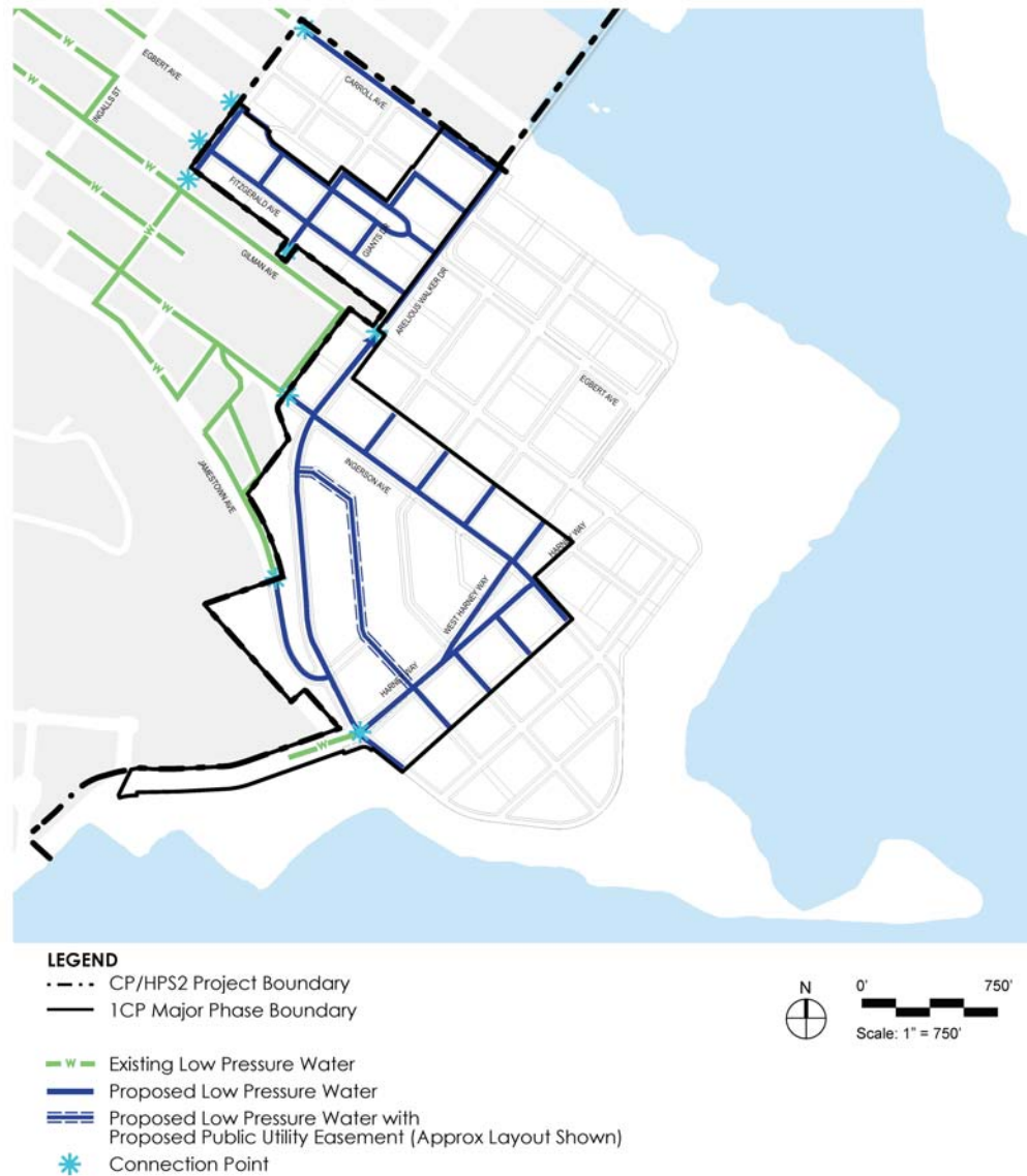
FIGURE 9.4: LOW PRESSURE WATER
