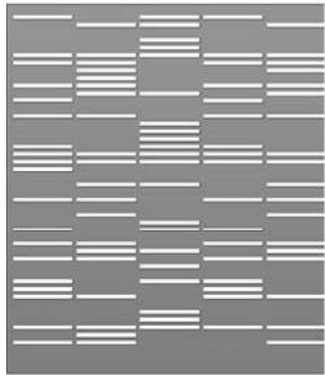
C SUNSHADES & RAILING: BOK METAL PANELS PERFORATED PATTERN B21 24% OPEN
