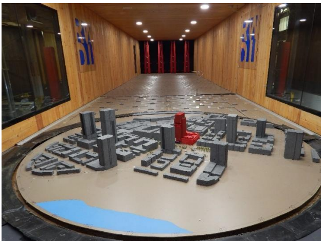
Image 2c: Wind tunnel study model – Existing + Project + Mitigation configuration
