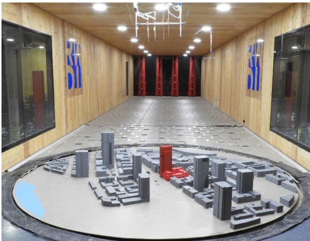
Image 2b: Wind tunnel study model – Existing + Project configuration
