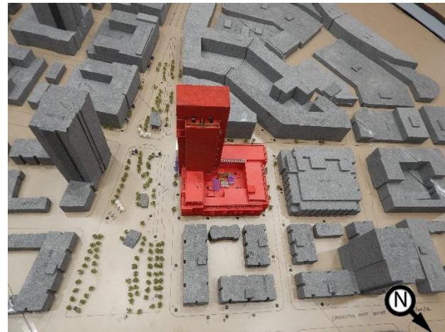
Image 2c: Wind tunnel study model – Existing + Project + Mitigation configuration
