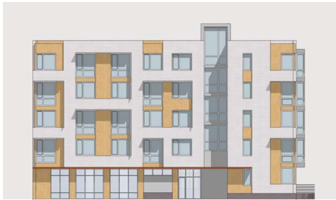
Coated metal window framing to match panels; clear low-e glass
