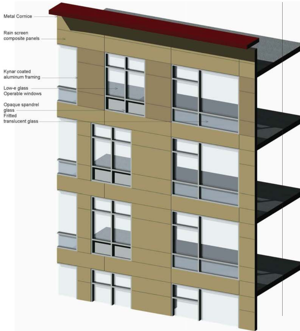
EXAMPLES: OPEN JOINT PANEL SYSTEM WITH STOREFRONT
